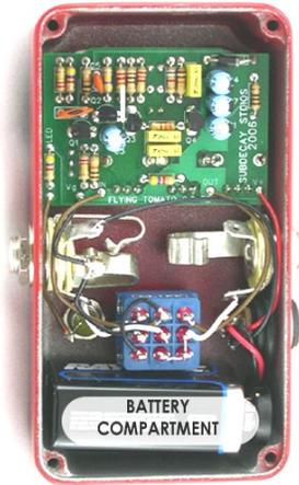
To change the battery first remove the 4 rear screws and the rear cover. The battery should be placed next to the switch in the battery compartment. The battery should be able to slide in and out with out any friction.
