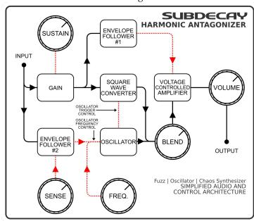
The square wave converter creates the fuzz sound. The oscillator is triggered for an effect similar to the sync function on a synthesizer. The voltage controlled amplifier keeps the output from hard gating as the input trails off.
