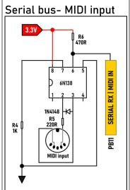
The 6N138 is recommended because it works well at 3.3v and 5v.
