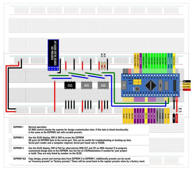
The BLUE & GREEN wire are the I2C bus. On startup EZ MIDI checks the bus for connected devices. If no devices are detected some versions of EZ MIDI may hang.
