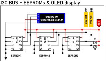
On power up EZ MIDI scans for I2C devices. Functionality is determined by what is connected to the I2C bus. If no devices are connected EZ MIDI may hang.
