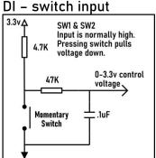
The 47K resistor and .1uF capacitor filters the switch signal to avoid noise and mis-triggers.
