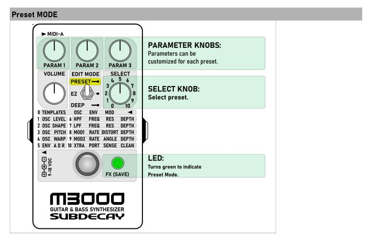
With the EDIT MODE switch set to PRESET use the select knob to load a preset.
