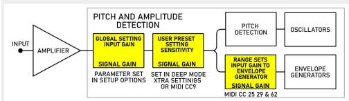
In short: Set the Global Gain for your guitar, then use Sensitivity per preset, and finally adjust the Range to shape how dramatic each effect is.
